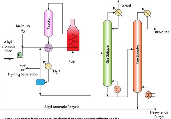
Note - For better heat economy in thermal process, reactor effluent can be used for stripper and fractionator reboiler heat supply.
